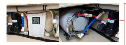
Connections at the ends of wires and splices in the middles are the most frequent points of failure for any wiring, especially in boats. Corrosion, stress, vibrations, and movement are the enemies here as well. ABYC standards are explicit. Also, electrical tape is not acceptable as a permanent wrap.
