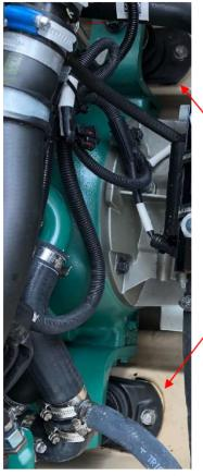
The engine mounts on this vessel transfer all of the thrust from the propeller via the propeller shaft through the transmission to the engine to the engine mounts into the hull stringers. For this reason, the condition of the engine mounts is critical.
